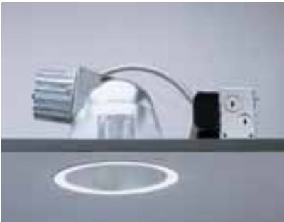
Lightolier "Calculite" compact fluorescent open downlight #8031 6" aperture triple tube horizontal lamp reflector trim: clear iridescence free, white flange available with electronic or dimming ballast available with emergency battery backup (508) 679-8131 or www.lightolier.com
