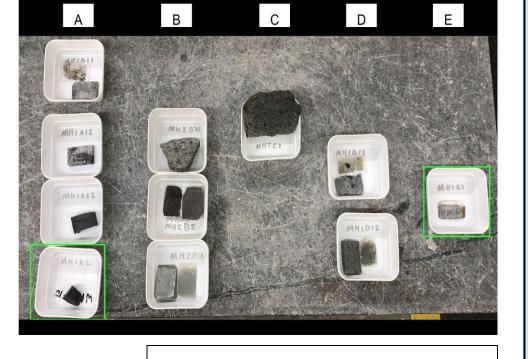
Figure 4: Samples that were used for comparative and thin-section analysis. Sample location from the column header relates to figure 2 locations. Green boxes indicate samples that were used for SEM.
