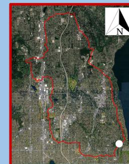
**Figure 4:** Thornton Creek basin showing a large amount of impervious surface shown by the grey areas. White dot displays the basin’s point of drainage. (StreamStats) (Imagery from Google Earth)
