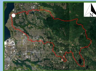
**Figure 3:** May Creek showing a moderate amount of impervious surfaces, left side mostly impervious, right side mostly forest. Point of drainage shown by white dot. (StreamStats) (Imagery from Google Earth)
