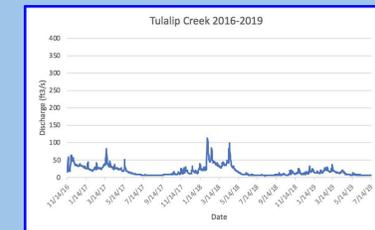
**Figure 9:** Detailed hydrograph for the least urban basin displaying a three year span to show clearer peaks and baseflows.
