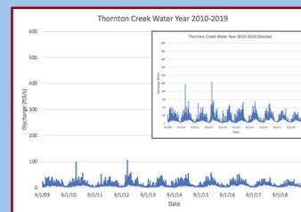
**Figure 7:** Hydrograph displaying the rate of discharge on a scale of 600 ft<sup>3</sup>/s as well as a scale of 200 ft<sup>3</sup>/s (to show more detail) during the span of nine years.
