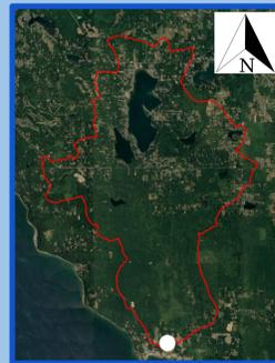
**Figure 2:** Tulalip Creek basin showing very little impervious surface due to amount of forestry (green areas) shown. White dot is displaying the point of drainage. (StreamStats) (Imagery from Google Earth)
