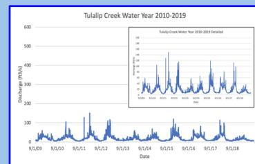
**Figure 5:** Hydrograph displaying the rate of discharge on a scale of 600 ft<sup>3</sup>/s as well as a scale of 200 ft<sup>3</sup>/s (to show more detail) during the span of nine years.
