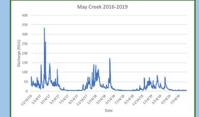
**Figure 8:** Detailed hydrograph for the second most urban basin displaying just a three year span to show clearer peaks and baseflows.
