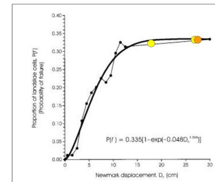
**Figure 4.** Weibull curve of Eq. 3 from Jibson et al. (2000). Demonstrates probability of slope failure as a function of Newmark displacement. Upper portion of curve indicates high probability of slope failure. Yellow and orange points are my results from Table 2 that were able to fit on the chart.
