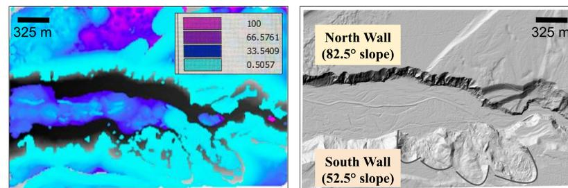
**Figure 3.** Factor of Safety output layer from Scoops 3D (left) and hillshade of study site (right). LiDAR image from Pierce DTM (2011). Light blue indicates a Factor of Safety range of 0.5057-10, lowest values in this range used for the Newmark Analysis. Differences in slope indicated.
