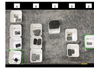
Figure 4: Samples that were used for comparative and thin-section analysis. Sample location from the column header relates to figure 2 locations. Green boxes indicate samples that were used for SEM.
