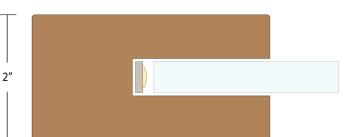
The 2"x4" frame will have a groove cut to insert the plexiglass and house the LED light strip. Because the LED light strip is wider than the plexiglass, the glass may need to be padded with adhesive foam.
