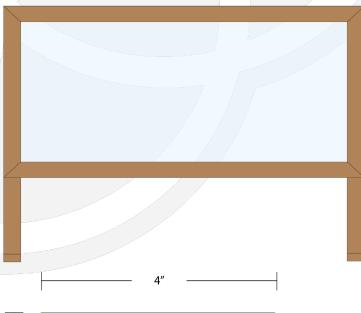
Front view of the lightboard. The board is clear Plexiglass acrylic sheeting. The standard size is 36"x72", but can be cut down, especially if there is a local plastic company you can purchase from. The glass should be at least .22 inches thick, to cut down on the amount of vibration that moves the glass when it's written on.
