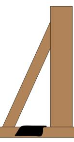
Side view of the leg construction. The legs are structured to brace the opposite side of the instructor, to counteract against the forward pressure of writing on the board. Sandbags help weight the legs down and stabilize the entire frame.
