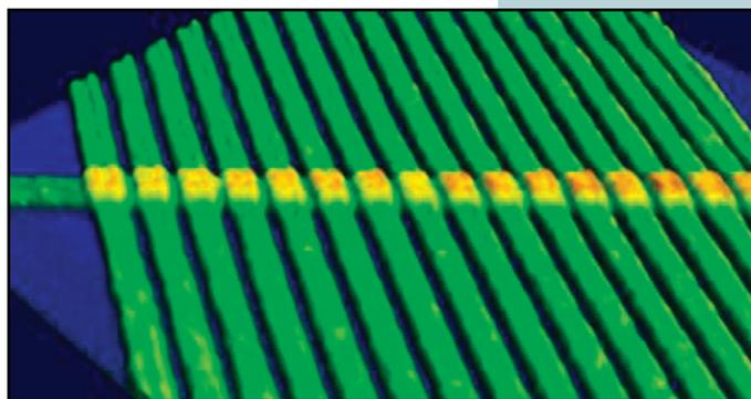
An array of 17 titanium oxide memristors, HP Labs
