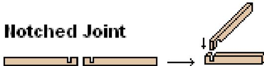
**Notched Joints** - the ends of the sticks have slits or notches cut into them and the notched ends slide together so that the sticks overlap.
