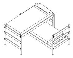
5. <u>Barrier Free Bed</u> Headboards are turned over. Rails use middle boring pattern. Mattress height is approx. 22"
