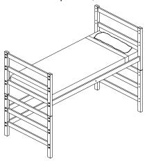
8. <u>High Loft</u> Rails on the back lower and top pattern for supporting frame.
