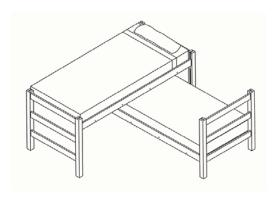
Steel side rails placed on **upper** set of pins for one bed.
