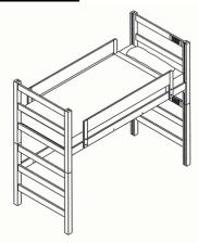
Steel side rails of bed placed on **bottom** set of pins.
