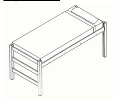
Steel side rails placed on **upper** set of pins.
