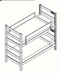
Steel side rails of top bed placed on **bottom** set of pins.
