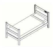
Steel side rails placed on **bottom** set of pins.
