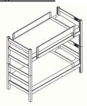
Steel side rails of the top bed placed on **middle** set of pins. Steel side rails of bottom bed placed on **lower** set of pins.
