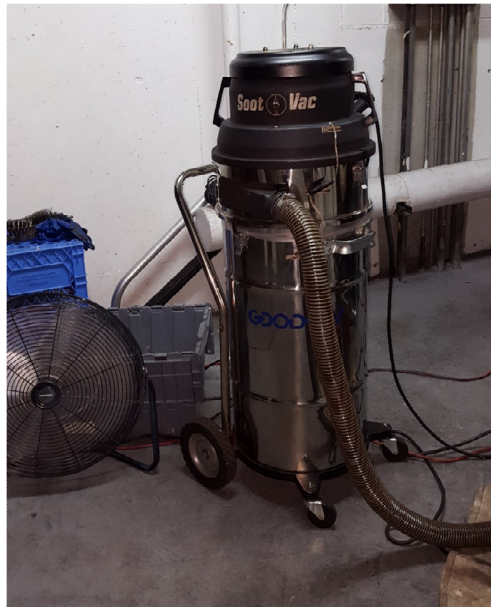
Photo 4, Goodway Model GTC-540 Soot Vac used for cleaning soot from boilers.
